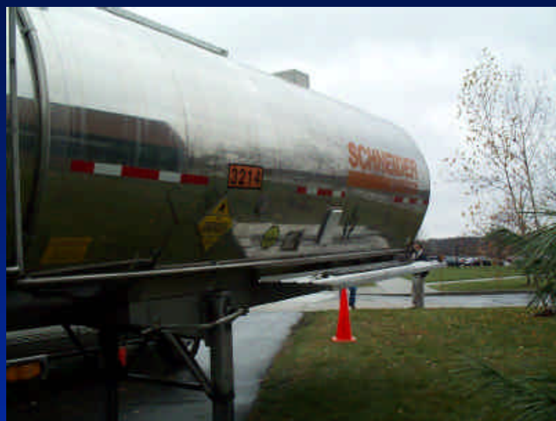
Two 5,000-gallon tanker trucks were used to transport and store sodium permanganate
